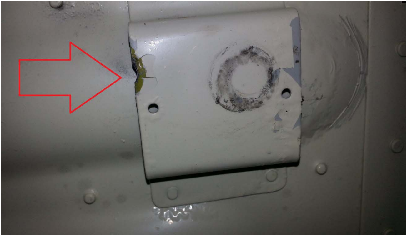
Figure 3 - MLG Up-Stop Bracket Wear
